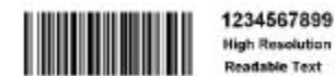
Figure 4: Typical bar code for a microplate label. 3 lines of human readable text are placed to the right of the actual Code 128 bar code.
